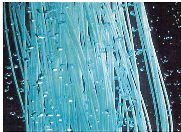
Figure 2. Hollow-fiber membranes (Image from GE/Zenon)
